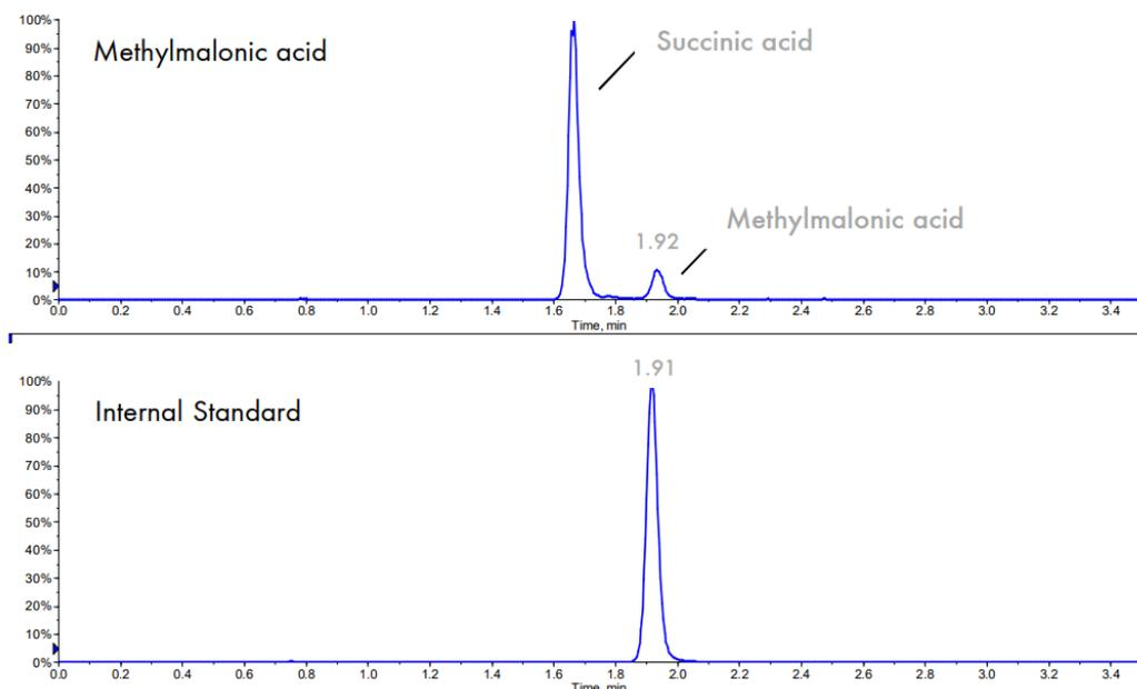
**Figure 3: The chromatographical separation of MMA and succinic acid.** The figure shows a representative chromatogram of a plasma calibrator with a MMA concentration of 254 nmol/L (kit insert MMA MassChrom reagent kit from Chromsystems).
