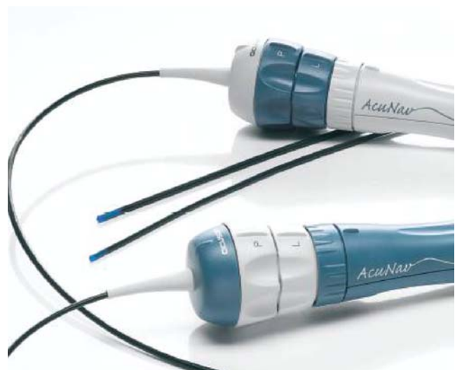
Fig. 1 Intracardiac echoprobes of 10 F and 8 F
