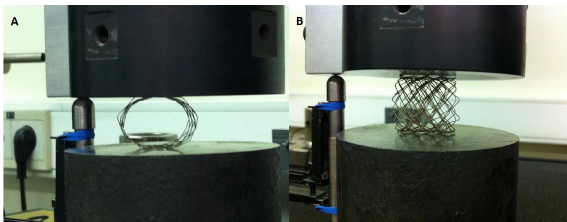
Figure 1. Compression bench testing. Instron bench testing demonstrated. A: Single CP stent, B: CP combination
