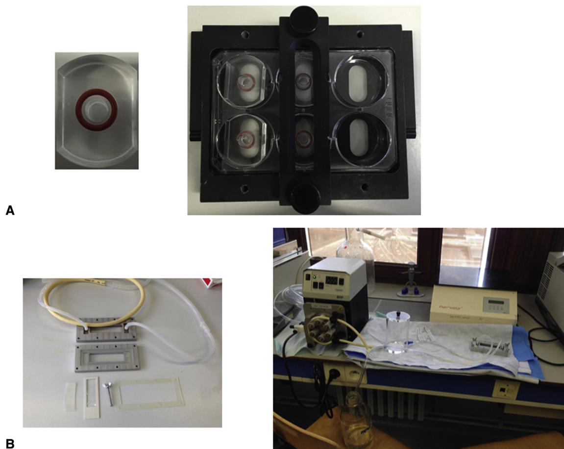
FIGURE E1. A, Image of the poly(methyl methacrylate) inlets with ring rubber gaskets (in-house design) mounted on a 6-well plate and fixed, using a metal frame (in-house design). B, Newly developed flow chamber (in-house design; Department of Tissue Engineering and Textile Implants, AME-Helmholtz Institute for Biomedical Engineering, Aachen, Germany) and the full installation for the bacterial perfusion.
