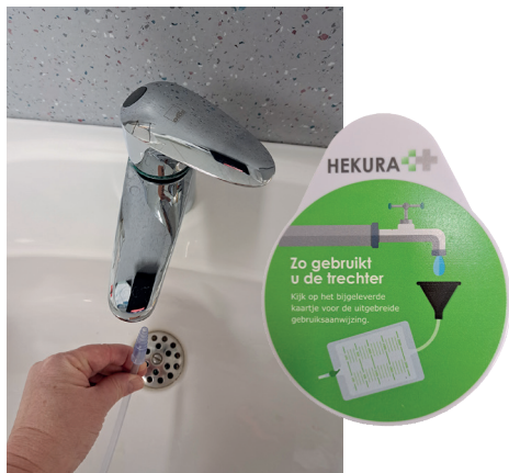
Figure 12. Let water run into the bag via the connector or using a funnel.
